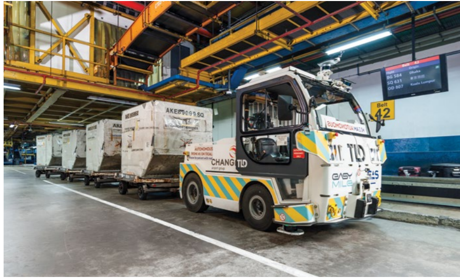
Autonomous tractor trials for baggage towing in conjunction with Changi Air Group
